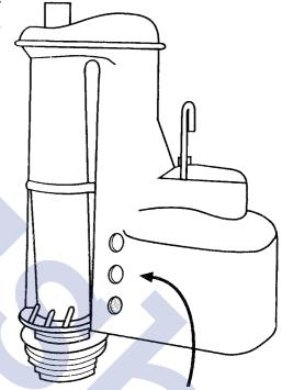
Press flush volume selector firmly into position to close the required holes.
